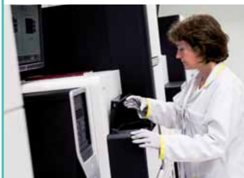
Installation of a flow cell containing prepared samples into a high-throughput sequencer (Illumina), in the Genoscope sequencer room.
