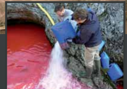
Injecting a tracer to monitor groundwater flow to characterize karst systems.
