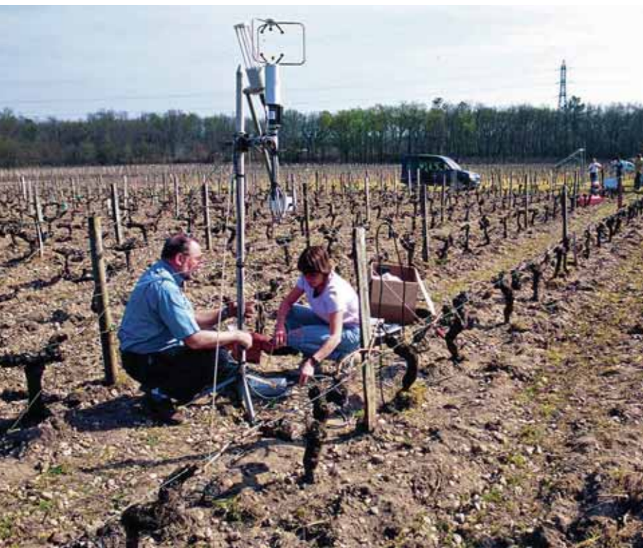
Installation of sensors in a Bordeaux vineyard to study the physical mechanisms that govern transfers between plant cover and the atmosphere.
