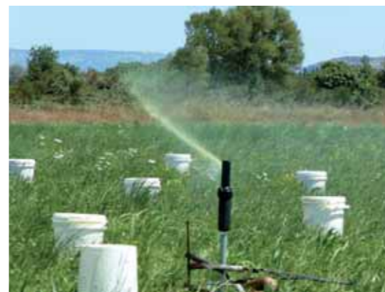
Assessing aerosol drift using a spray system and water with a coloring agent added to simulate wastewater.
